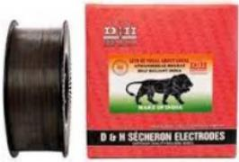
LoTherme OA-617 is a hard-surfacing wire to deposit complex carbides of chromium, molybdenum along with niobium and tungsten. The weld metal has excellent abrasion resistance property for low impact applications at service temperature up to 600°C. The deposited weld bead has metallic appearance and does not require any post-weld cleaning. Stress relief cracks appear on surface of the weld during cooling of the bead. Weld bead is machinable by grinding.
