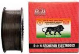
LoTherme OA-602 is a wire to deposit low alloy air-hardening type weld metal having moderate resistance to abrasion and very good resistance to impact & compression. The wire is suitable for rebuilding of carbon & low alloy steel components where resistance to compressive loading is of prime importance. It is also used as a buffer layer prior to hard surfacing.
