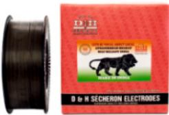
A basic type medium alloy gas shielded wire designed for air hardening type hard surfacing deposit. It has good welder's appeal & easy slag detachability. The weld is non-machinable and finished by grinding. The wire deposits a crack-free, martensitic weld metal suitable for heavy impact and moderate abrasion resistant applications.
