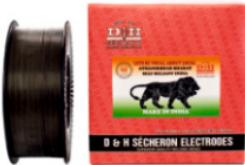
A basic type high alloy gas shielded flux cored wire designed for air hardening type hard surfacing deposit for severe abrasion resistant applications. It has good welder's appeal & easy slag detachability. The weld is non-machinable and finished by grinding. The wire deposits a crack-free, martensitic weld metal that can impart excellent resistance to mineral wearing stresses and abrasion.
