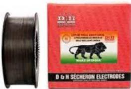
LoTherme OA-611 (SPL) is a hard-surfacing wire to deposit a superior distribution of chromium carbides in a martensitic matrix. The weld metal has excellent abrasion resistance property and has good corrosion & erosion resistance in mineral-water mixer. Suitable for hard surfacing of MS Plate for Wear Plate. Weld deposits reveals stress relief cracks during cooling of the bead and is machinable by grinding only.
