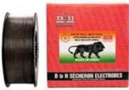
LoTherme OA-611 is a hard-surfacing wire to deposit chromium carbides having excellent abrasion resistance property even for elevated temperature applications. The weld metal has good corrosion & erosion resistance in mineral-water mixer. Weld reveals stress relief cracks during cooling of the bead. Weld metal is machinable by grinding only.
