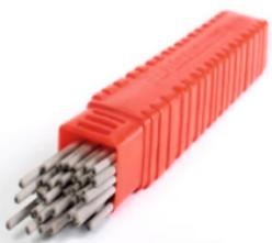
LoTherme-355 is an extra low hydrogen low heat input electrode depositing a low alloy steel, high strength weld metal ideal for maintenance and repair welding of Cr - Ni - Mo high strength low alloy steels, case hardened steels, heat-treated steels, etc. The extra low hydrogen helps in preventing cold cracks.
