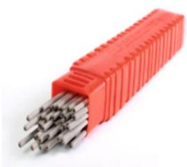
LoTherme-410 is a low heat input, high deposition electrode, depositing air-hardening type chromium steel having 12.5% Cr. The weld deposit displays good resistance to corrosion, erosion, pitting and abrasion.
