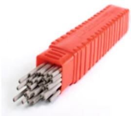
LoTherme-464 is characterized by a stable arc, which is easy to strike and re-strike. Easily removable slag, smooth finely rippled welds of radiographic quality. The weld metal is fully austenitic in structure and possesses high strength, high ductility, good toughness and creep strength. Resistance to scaling is retained up to 1200°C.
